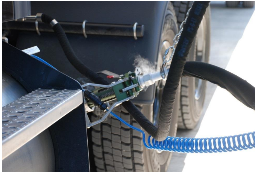
Figure 10: LNG Fueling: 3 hoses- fuel, pressure relief, and electrical ground; Source: CCBR
