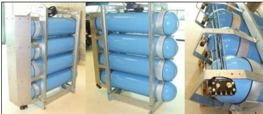
Fig 26: Prins 4 x 140L vertical CNG cylinder pack
