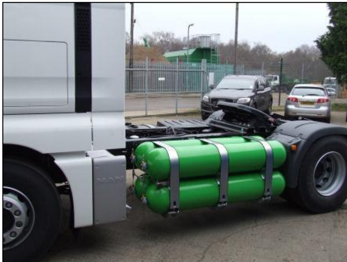
Fig 24: Prins dual-fuel conversion (MAN)
