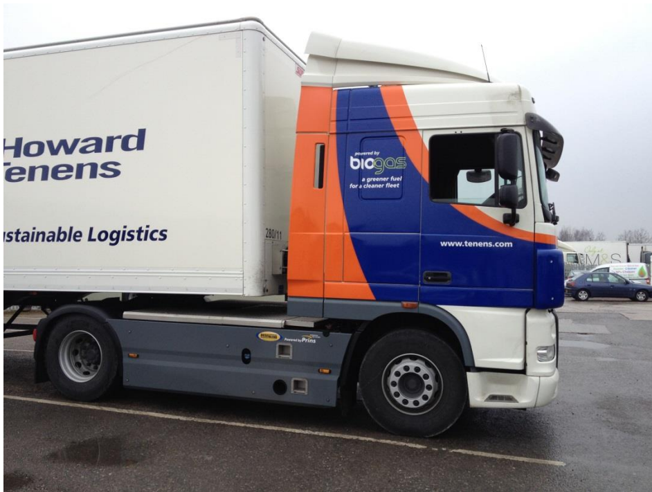
Fig 25: Prins dual-fuel conversion (DAF)
